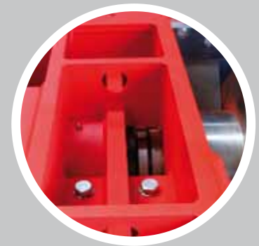
Bearings outside the cutting chamber
